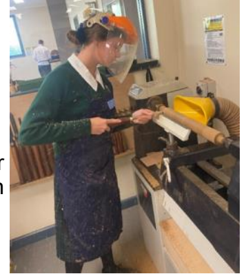
Hayley Wilson uses the wood lathe to work on her French rolling pin
